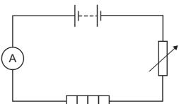
The variable resistor is adjusted until the reading on the ammeter is 0.50 A and the resistance of the heater is  $8.0\,\Omega$ .
